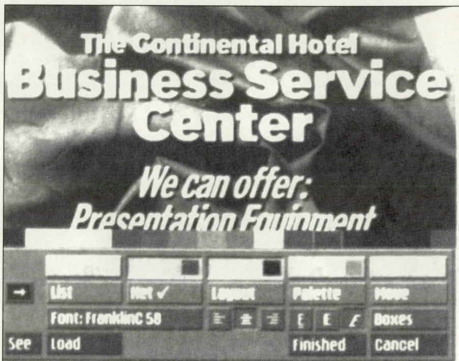
Scala's editing menu. All editing of text and symbols are controlled from this menu. Submenus include typography, colour control, transitions and text import.
