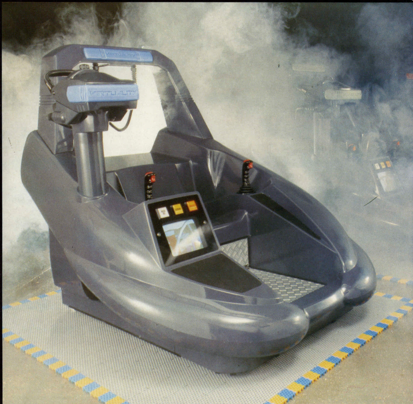
Virtuality 1000SD, a high quality, sit down console which enables the operator to drive his "vehicle" in a virtual world.
