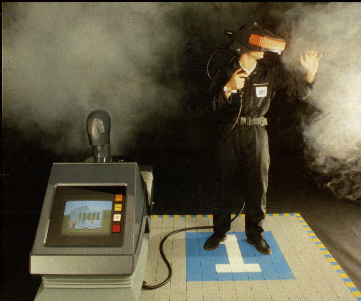
The Virtuality 1000 SU designed for a user standing or moving within a scanned area, with the VIssette visor providing an interface with the virtual world. Interaction with the virtual world is provided by a hand-held unit.
